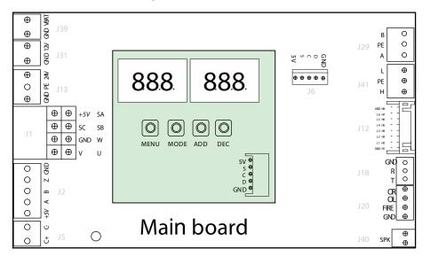
There are 4 keys on the main motor driving controller, "MENU", "MODE", "ADD" and "DEC".
